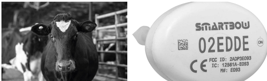
Images 1-2: Dairy cow fitted with SMARTBOW ear tag behaviour monitor (Left) and close up of the SMARTBOW ear tag (Right).
