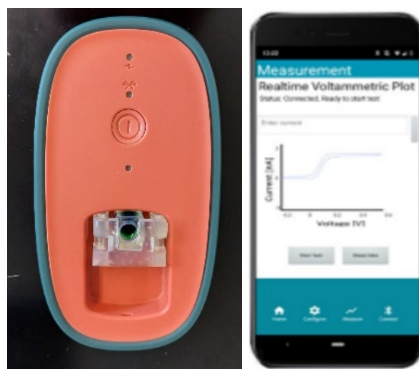
Images 3-4. Example of a point-of-care (hand-held) sensor that could allow analytes in milk to be rapidly detected (Left) and display of sensor reading on a smartphone (Right).
