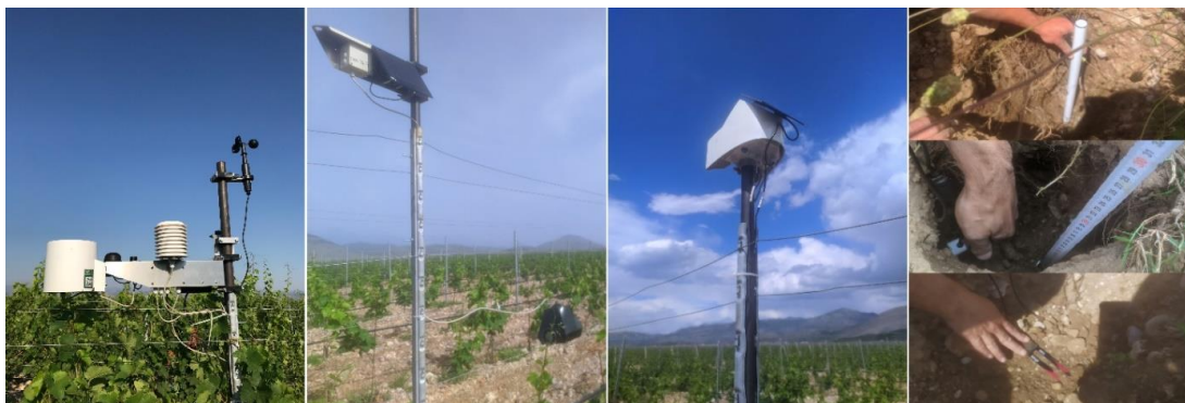
Figure 30 Pictures of the sensor nodes installed at the pilot site, from left to right: a) weather station; b) digital pheromone insect trap with camera, c) soil moisture node; d) three types of soil moisture sensors.
