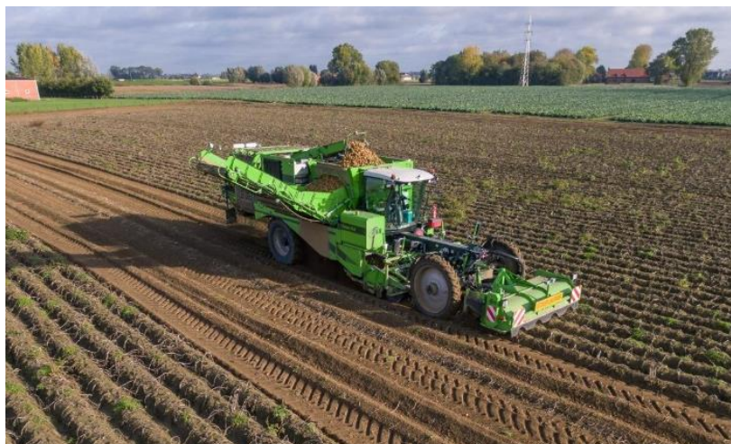
Figure 38: AVR Puma 4.0 potato harvester with GPRS/4G data connection
