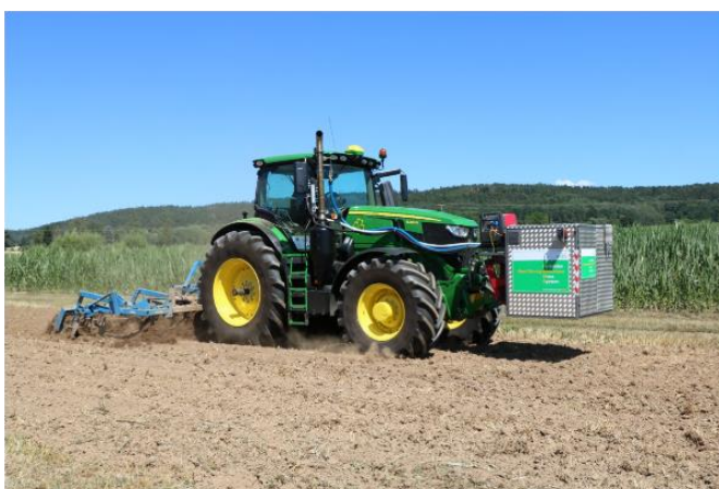
Figure 19: Emission measurement system
