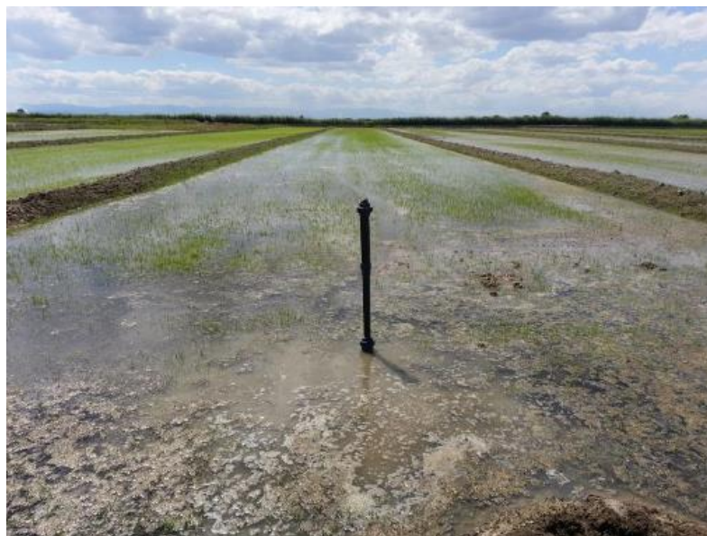
Figure 57: Prototype of the salinity sensor Smart-Paddy, that was placed in a rice field of experimental station of Kalochori of ELGO in 2013.
